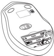
Fig. 6. Fitting the receiver into the mouse case
