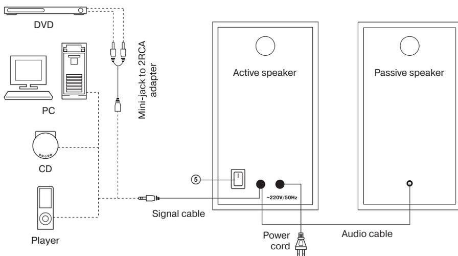
Fig. 2. Connection diagram
