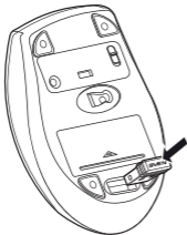
Fig. 6. Fitting the receiver into the mouse case
